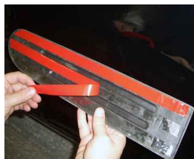
4. Peel off the release liner
