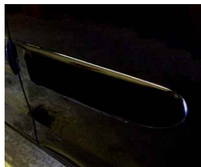
6. The Bodyside moulding is now securely fixed to the vehicle
