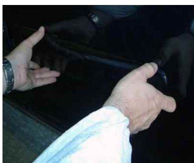
5. Position the moulding and apply pressure onto the panel applying pressure evenly over the moulding ensuring it is well secured
