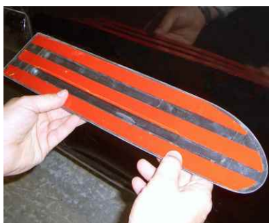
3. Apply the Acrylic tape to the body moulding and apply pressure evenly over the tape
