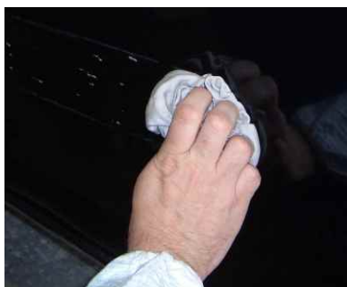
1. Clean and degrease the panel where the body moulding is to be applied
