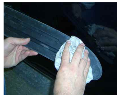
2. Clean and degrease the body moulding
