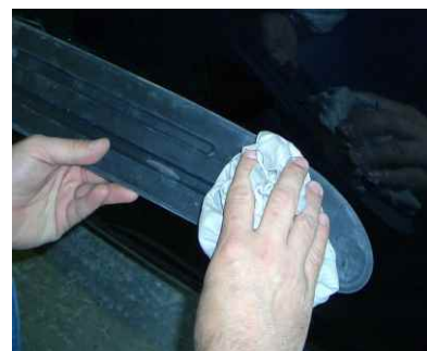
2. Clean and degrease the panel body moulding
