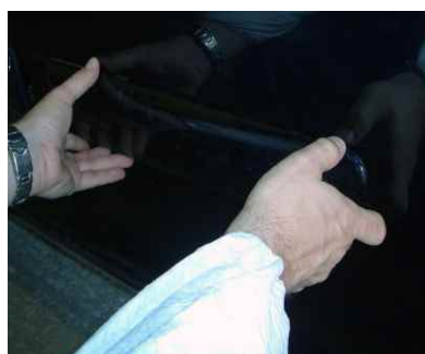
5. Position the moulding and apply onto the panel applying pressure evenly over the moulding ensuring it is well secured
