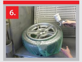
6. To complete the masking process, flip the wheel over, checking that the elasticated band is still creating a seal and then paint.
