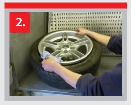
2. Before masking the wheel, clean the inner rim ensuring it's free from dirt and grease.
