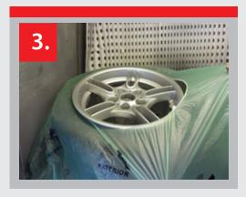
3. Apply the product by placing the elasticated band around the rim, ensuring the treated side of the film is facing upwards.
