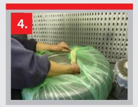
4. When you have positioned the product into place, carefully flip the wheel over so the alloy is facing the ground, draw the corners of the product together & tape down.
