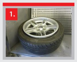
1. Remove wheel from the vehicle & deflate the tyre.
