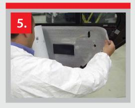
5. Once you have finished cutting the shape out, you are now ready to fit to the car. Peel off the release liner to expose the adhesive. Position this on the door taking care to ensure it is in the correct position. Press it firmly in place.
