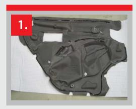
1. Pull out enough material out of the dispensing box. Lay on a flat surface with the paper grid side face up. If possible lay the old door skin film over the top.
