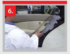
6. Replace the inner door panel and fix all the interior parts back onto the car.
