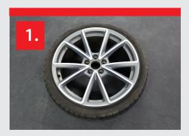
1. Remove wheel from the vehicle and deflate the tyre.
