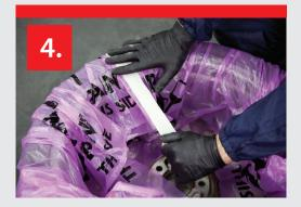
4. Carefully flip over so the wheel is facing the ground, draw the corners of the product together and tape down.
