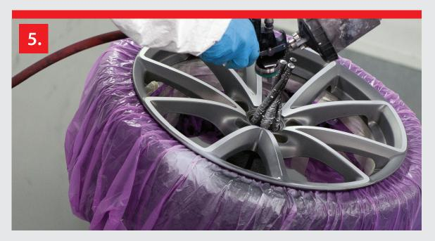
5. To complete the masking process, flip the wheel over, checking that the elasticated band is still creating a seal and then paint.
