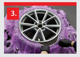
3. Apply the product by placing the elasticated band around the rim, ensuring the treated side of the film is facing upwards.
