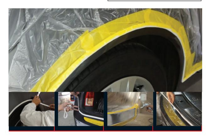
A flexible product designed to mask curved swage lines & panel edges. Eliminates unnecessary rework.
