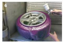
To complete the masking process, flip the wheel over, checking that the elasticated band is still creating a seal and then paint.
