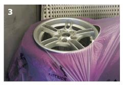
Apply the product by placing the elasticated band around the rim, ensuring the treated side of the film is facing upwards.
