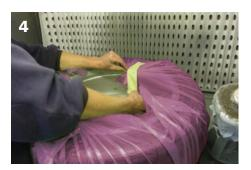
When you have positioned the product into place, carefully flip the wheel over so the alloy is facing the ground, draw the corners of the product together & tape down.
