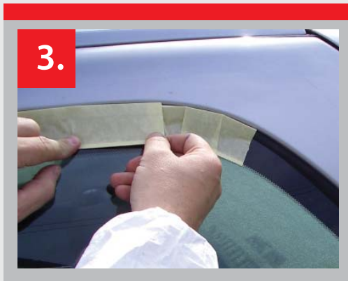
3. To mask along a straight section, tear off a section no longer than 20cm, slide in and leave back the trim ensuring it overlaps the last piece.
