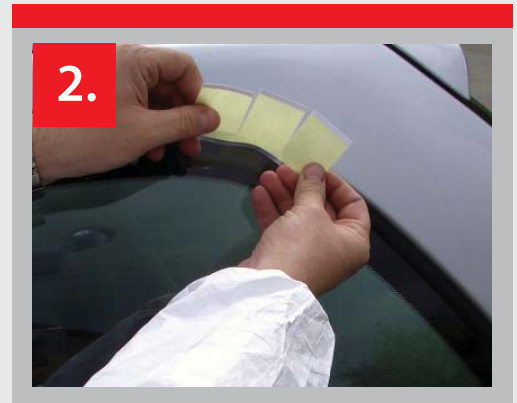
2. Tear off a small section to mask a tight corner and tear the tape down to the plastic section. Then slide in between the rubber trim and bodywork.
