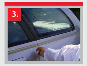
3. Select the stripe configuration and pull out desired sections. Press the tape firmly down along the length.
