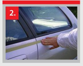
2. Apply the tape onto the vehicle and apply light pressure.
