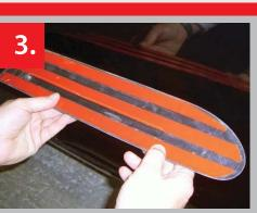
3. Apply the acrylic tape to the body moulding and evenly apply pressure onto the tape.
