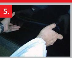
5. Position the moulding and position onto the panel applying pressure evenly over the moulding ensuring it is well secured.
